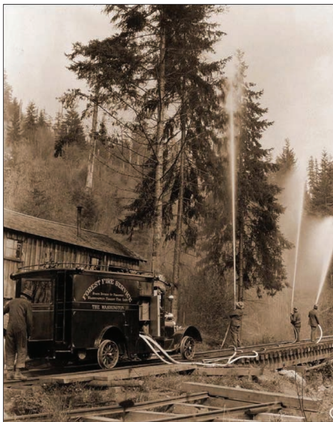
WFFA developed a fire truck capable of riding on both rail and road.
